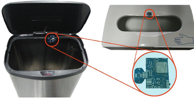
Fig. 3. Dummy nodes located in trash can and gloves dispenser.
